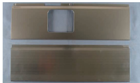
Figure 7 Aluminum extruded shape. Upper: As hairline treated. Lower: As extruded.
