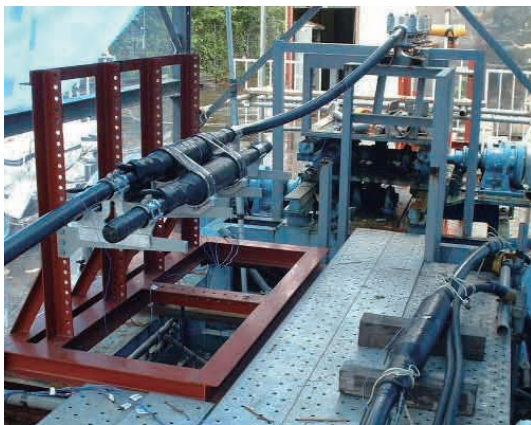
Figure 2 Testing set-up for offset section loading test.
