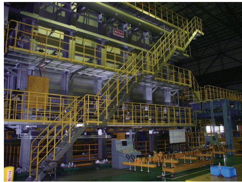
Figure 2 No.2 quenching furnace.
