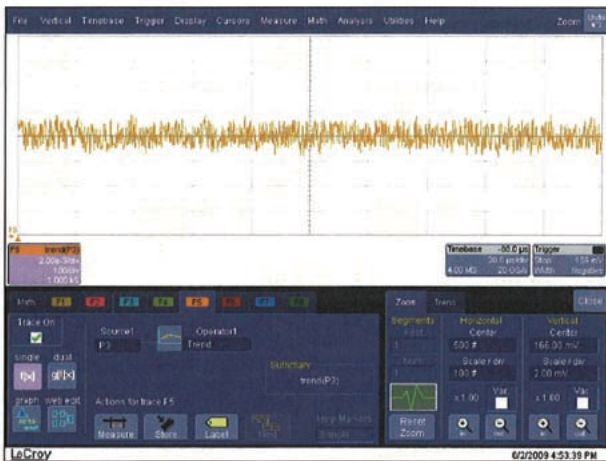
Figure 13 Trend chart of optical average launch power at the beginning of each burst span.
