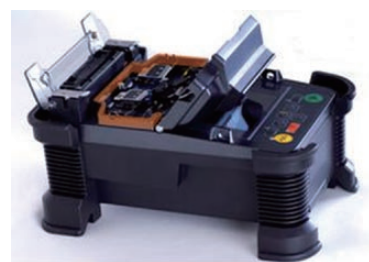
Figure 6 Canopy and top case structure for wind protection.
