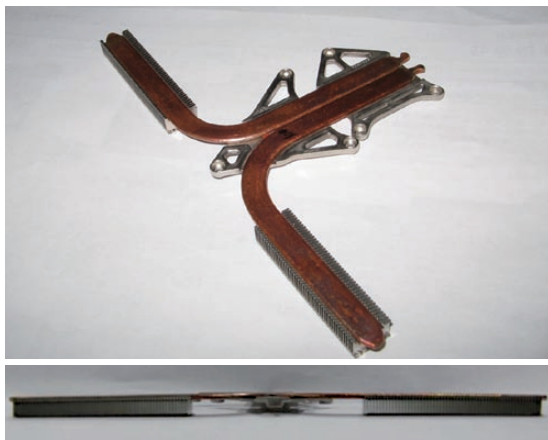
Figure 5 Thin heatsink with heatpipe and fin. (Two heatpipes with thickness of 2 mm are used, for 50 W CPU.)
