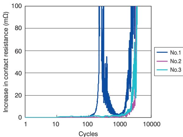
Figure 3 Profile of contact resistance on fretting test.
