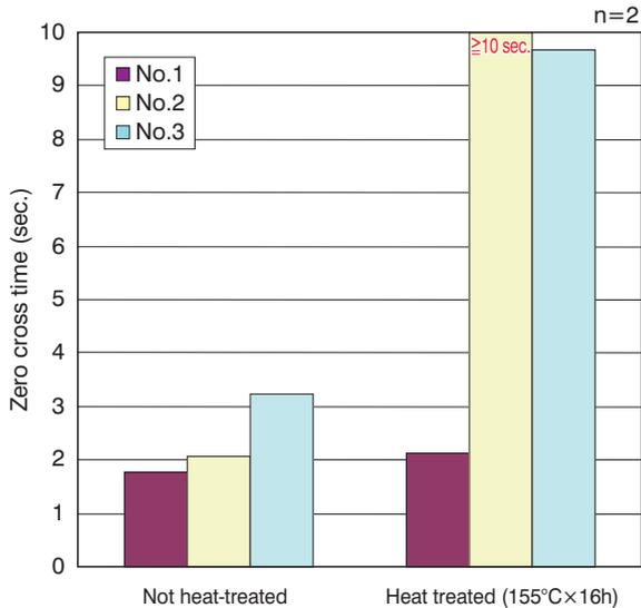
Figure 6 Wetting time of Sn-3Ag-0.5Cu solder.
