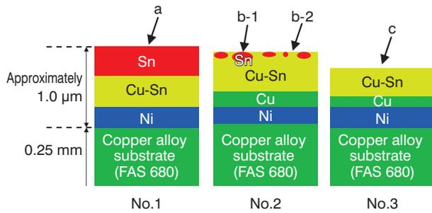
Figure 1 Section images of the plating samples.
