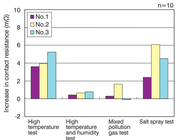
Figure 5 Contact resistance after the environmental tests.
