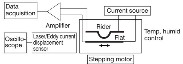
Figure 2 Schematic view of the fretting experiment tester.
