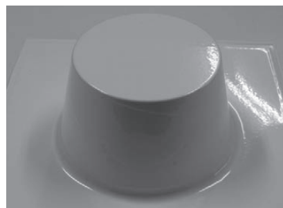
Figure 4 Vacuum and pressurized air forming sample of MCPOLYCA.
