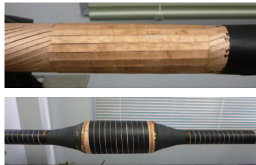
Figure 5 Normal joint of HTS for the over-current test.
