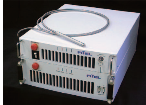
Figure 1 Air-cool-type fiber laser with 300 W output. (Upper: power supply, Lower: optical section)
