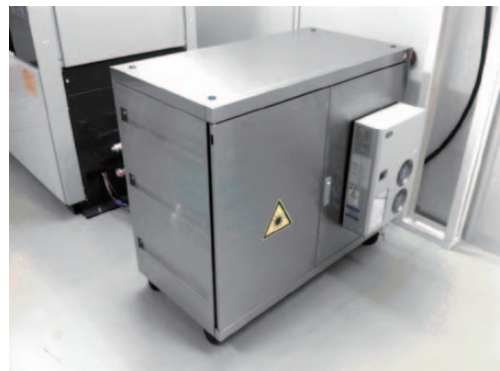
Figure 6 Fiber laser with 2 kW output.
