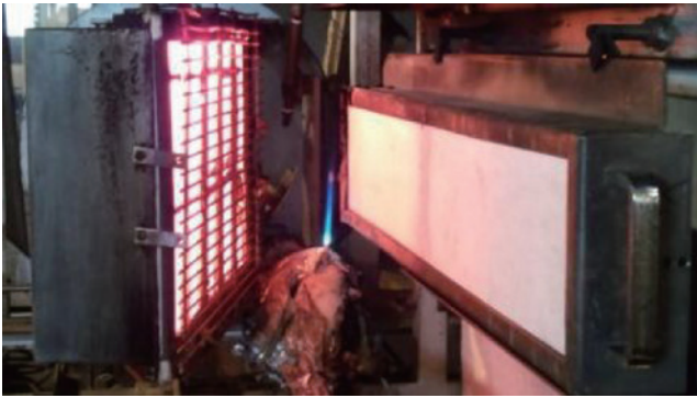
Figure 3 Flame propagation testing equipment, the heating part (Left) and the ignition panel (Right).
