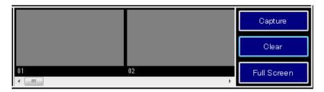
The screen image is zoomed by clicking [Full Screen]. In the full screen mode, because the control buttons are not displayed, use the key of the fusion splicer. The screen returns to original size by clicking [Back].
