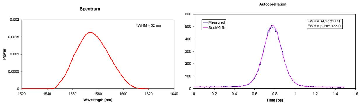
Figure 2. Left: Output spectrum of oscillator. Right: Autocorrelation trace form oscillator after compression in 3.6 m SSMF
