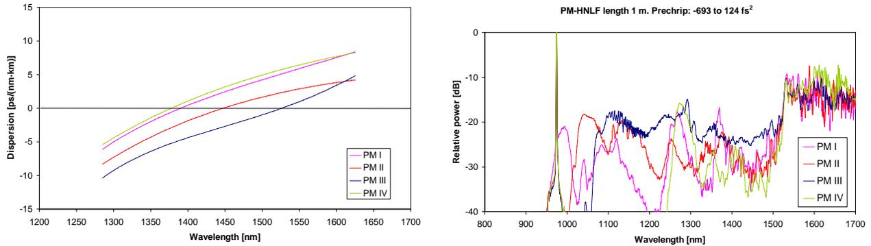
Figure 8. Left: Dispersion profile for four PM-HNLFs. Right: Measured supercontinuum spectra on 1 m of PM-HNLF.
