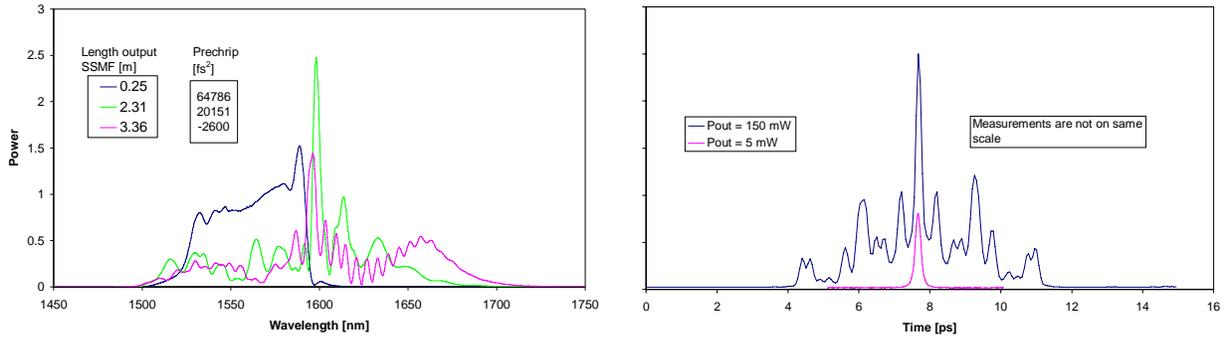
Figure 3. Left: Amplifier output spectrum at 150 mW output power. Right: Amplifier autocorrelator traces after prechirping in 3.24 m SSMF.
