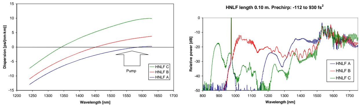
Figure 5. Left: Dispersion profile for three HNLFB. Right: Measured supercontinuum spectra on 0.1 m of HNLFB.
