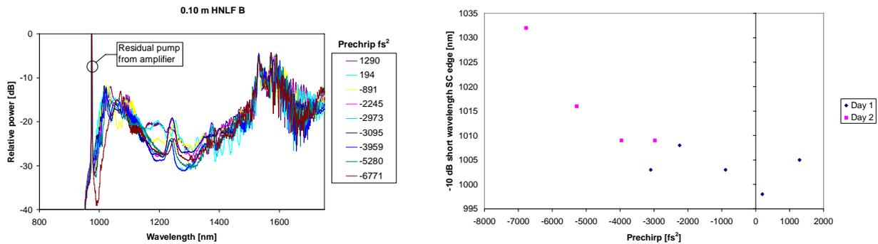
Figure 4. Left: Measured supercontinuum spectra for different prechirp. Right: -10 dB short wavelength supercontinuum edge as a function of prechirp.
