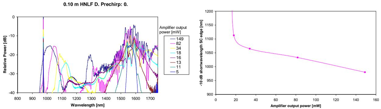
Figure 7. Effect power. Left measured supercontinuum spectra. Right: short wavelength supercontinuum edge as function of pump power.
