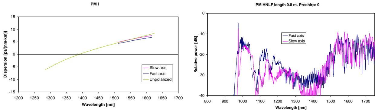
Figure 9. Left: Dispersion profile for PM-HNLF I. Right: Measured supercontinuum spectra on 0.8 m of PM-HNLF
