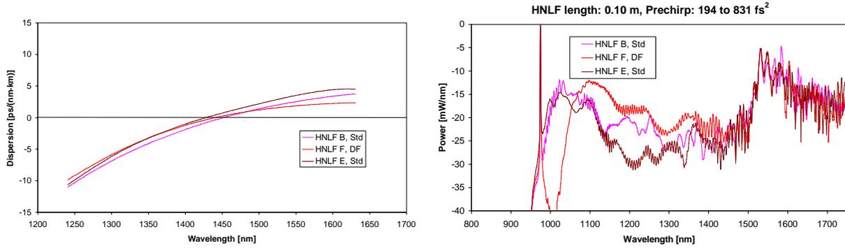
Figure 6. Left: Dispersion profile for three HNLF. Right: Measured supercontinuum spectra on 0.1 m of HNLF.
