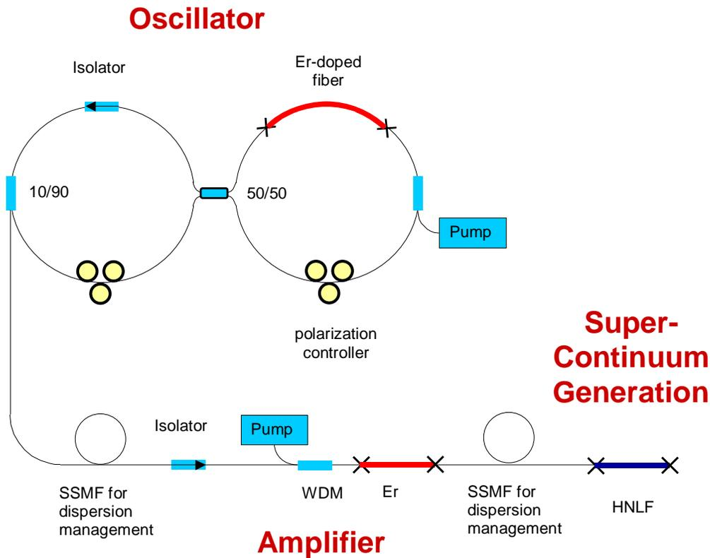
Figure 1. Experimental setup with figure 8 oscillator, and amplifier. Dispersion between stages is managed by length of SSMF.
