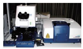
FT-IR: Fourier-Translation Infrared Spectroscopy (elemental analysis for organic compound)
