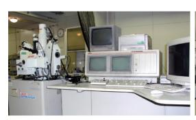
EPMA: Electron Probe Micro-analyzer (structural and composition distribution analysis)
