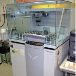
XRF:X-ray Fluorescence Analysis (elemental analysis)
