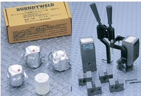
Copper thermite materials and crucible for welding
