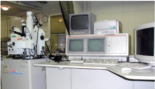
EPMA: Electron Probe Micro-analyzer (structural and composition distribution analysis)
