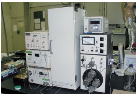
HPLC: High Performance Liquid Chromatography (qualitative and quantitative analysis for liquid)
