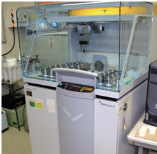
XRF: X-ray Fluorescence Analysis (elemental analysis)
