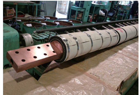
An exterior view of the water cooled cable in the process of manufacturing
