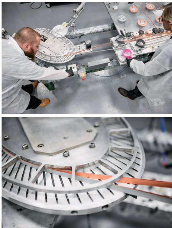
Figure 1 The HTS magnet for compact fusion reactor developed by Tokamak Energy Ltd.
