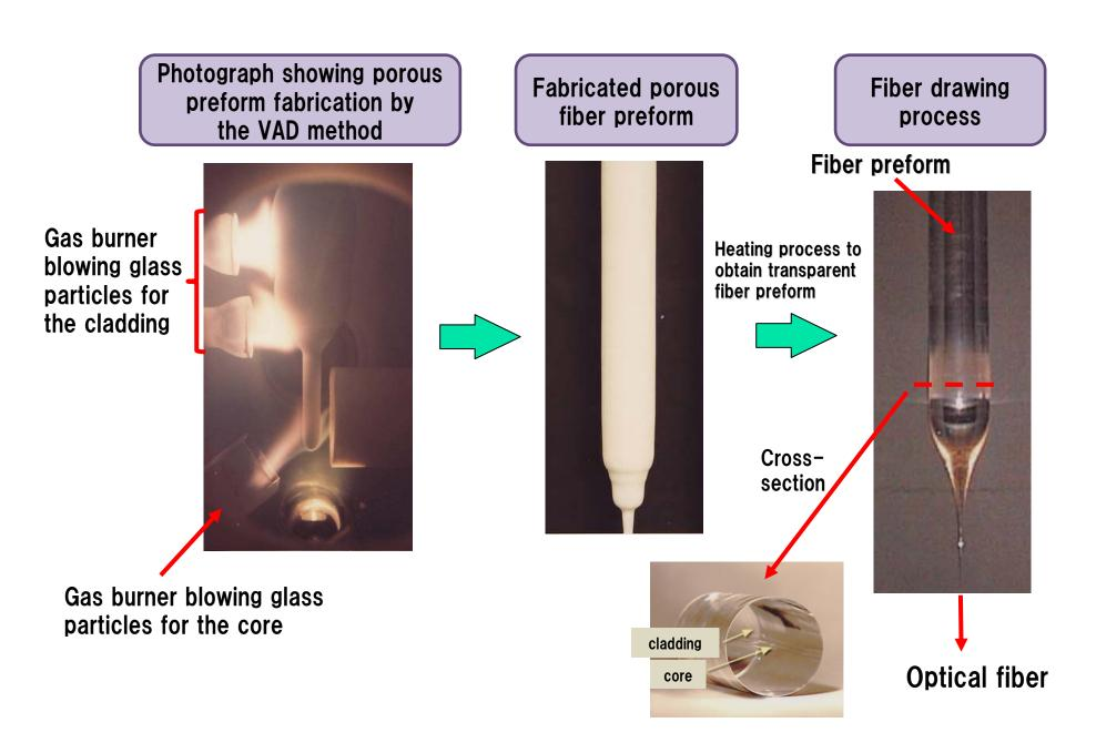
Figure 1 Optical fiber fabrication by the VAD method.
