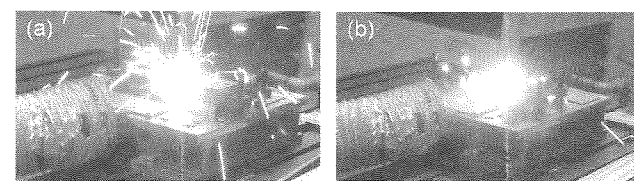
Fig. 10 Images of spattering of bead-on-plate of stainless steel using (a) conventional single spot and (b) beam mode control.
