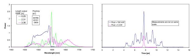
Figure 3. Left: Amplifier output spectrum at 150 mW output power. Right: Amplifier autocorrelator traces after prechirping in 3.24 m SSMF.
