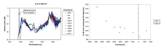
Figure 4. Left: Measured supercontinuum spectra for different prechirp. Right: -10 dB short wavelength supercontinuum edge as a function of prechirp.
