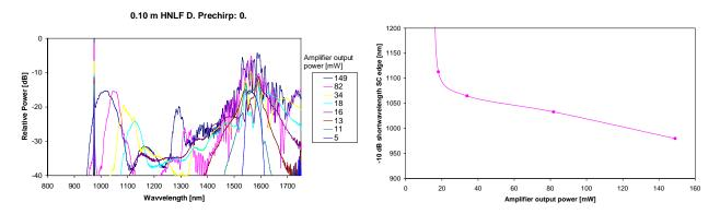
Figure 7. Effect power. Left measured supercontinuum spectra. Right: short wavelength supercontinuum edge as function of pump power.
