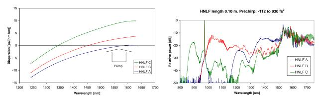
Figure 5. Left: Dispersion profile for three HNLF. Right: Measured supercontinuum spectra on 0.1 m of HNLF.
