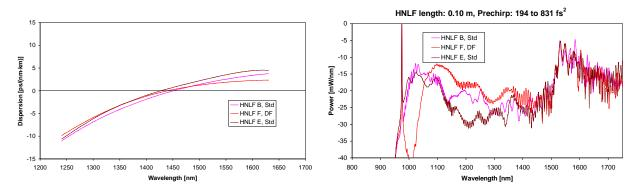
Figure 6. Left: Dispersion profile for three HNLF. Right: Measured supercontinuum spectra on 0.1 m of HNLF.
