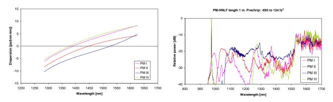
Figure 8. Left: Dispersion profile for four PM-HNLFs. Right: Measured supercontinuum spectra on 1 m of PM-HNLF.
