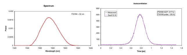
Figure 2. Left: Output spectrum of oscillator. Right: Autocorrelation trace form oscillator after compression in 3.6 m SSMF
